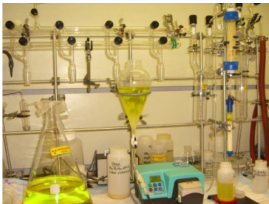
Demonstration of the separation of uranium from technetium for fuel cycle application
