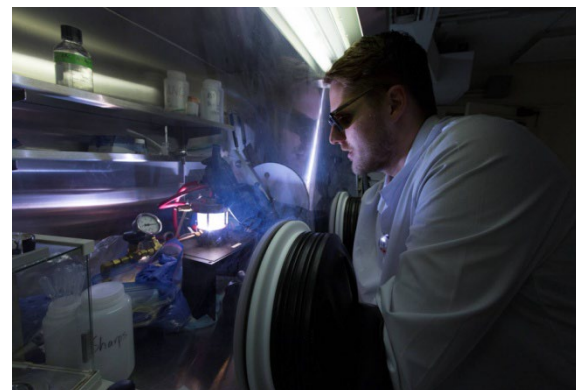
Preparation of U-Tc alloys by arc melting
