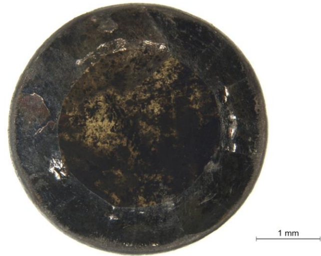
Natural diamond with CO 2 inclusions at a pressure of 20000 atmospheres
