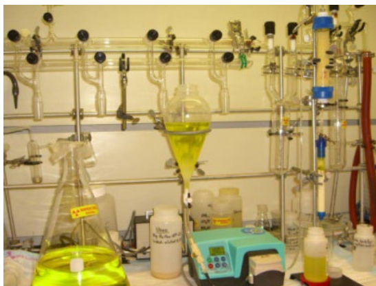
Demonstration of the separation of uranium from technetium for fuel cycle application
