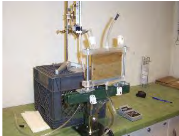
Hydraulic conductivity of a rock slab
