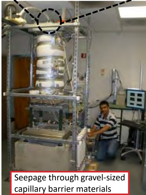
Millimeter-scale transport experiment
