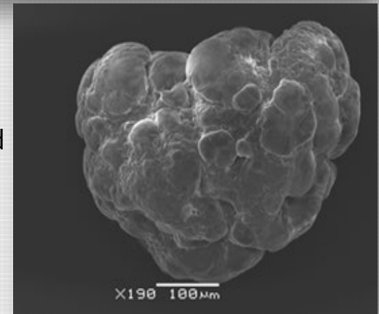
A microfluidic system designed for biofilm investigation in space (top left); Silk fibroin porous particles created by the Ouzo effect.
