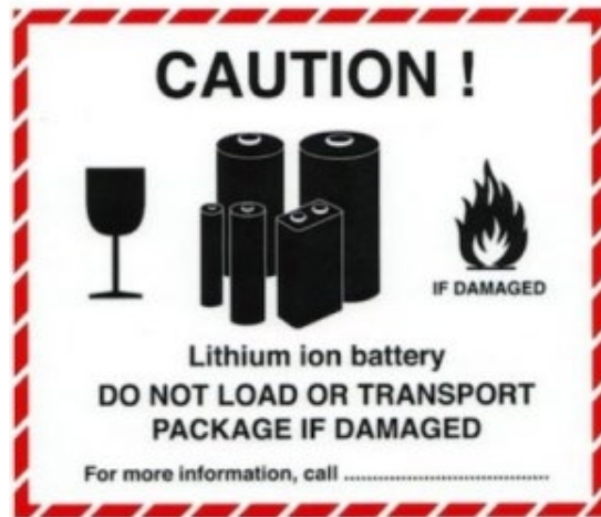
Figure 3. Mandatory label for lithium ion battery shipments that fall below DOT thresholds for Hazardous Materials labeling
