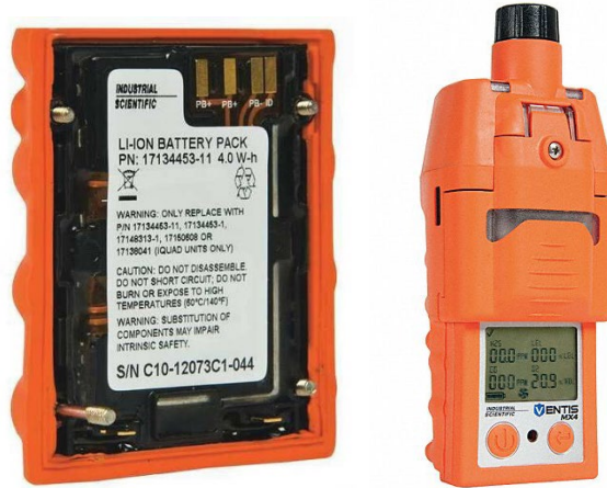
Figure 2. Example of lithium-ion batteries that are packed with, or contained in, the equipment they power. At energy levels of <100 W-h per battery pack or 20 W-h per cell, these are exempt from Dangerous Goods shipping requirements.
