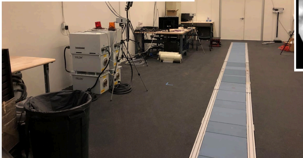
Gait laboratory for force and x-ray motion analysis of canine gait
