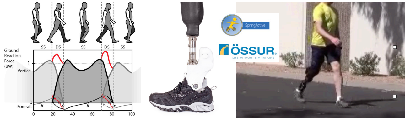
Ground reaction forces are measured to determine dynamics in every instance of the stride
